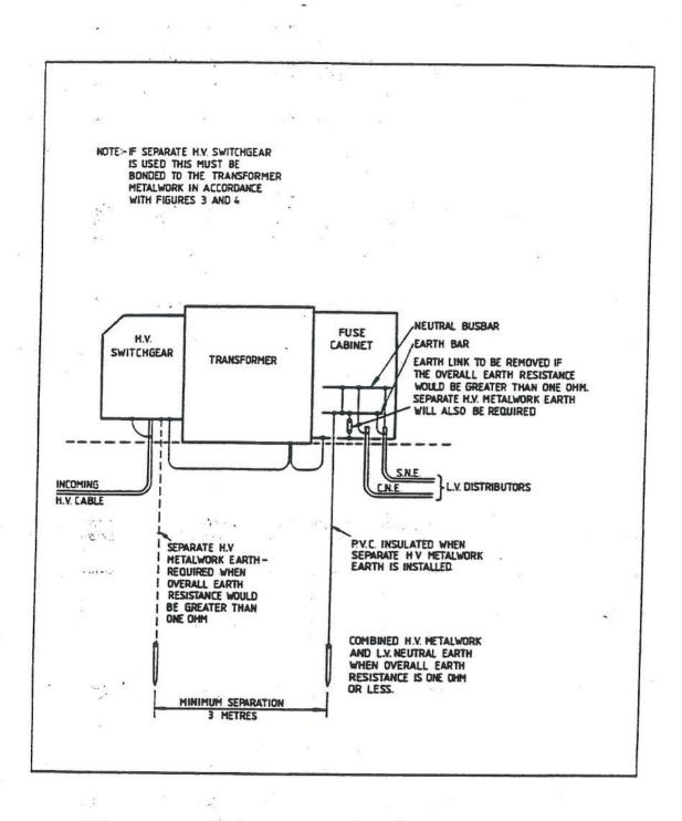
FIGURE 5: GROUND MOUNTED SUBSTATION WITH TRANSFORMER MOUNTED FUSE CABINET
