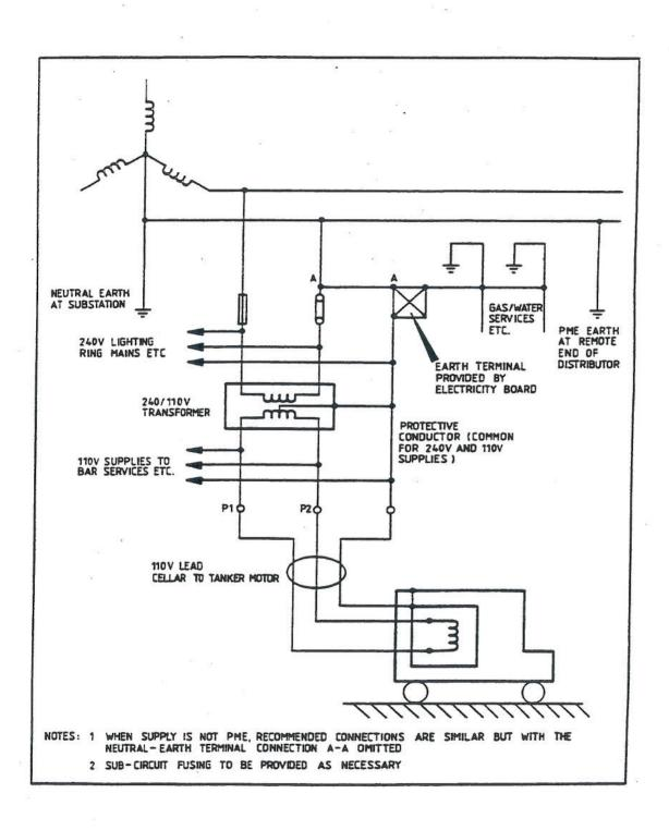
FIGURE 7: RECOMMENDATIONS FOR CONNECTIONS OF 240V AND 110V INTERNAL DISTRIBUTION WHEN SUPPLY IS PME
