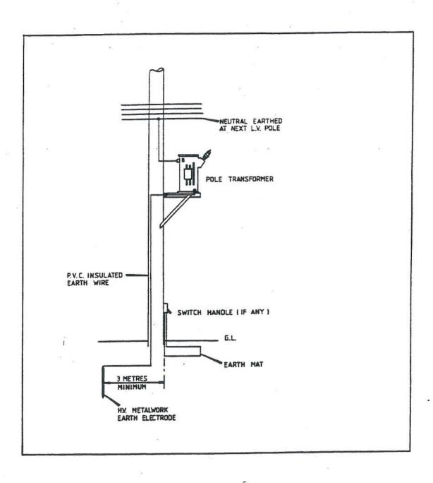
FIGURE 1: POLE TRANSFORMER FEEDING OVERHEAD LINE
