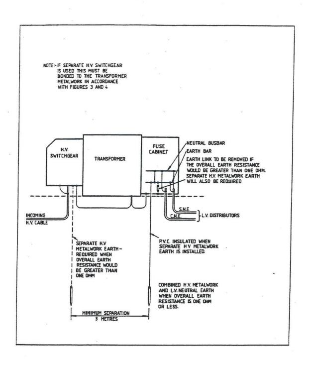
FIGURE 5: GROUND MOUNTED SUBSTATION WITH TRANSFORMER MOUNTED FUSE CABINET
