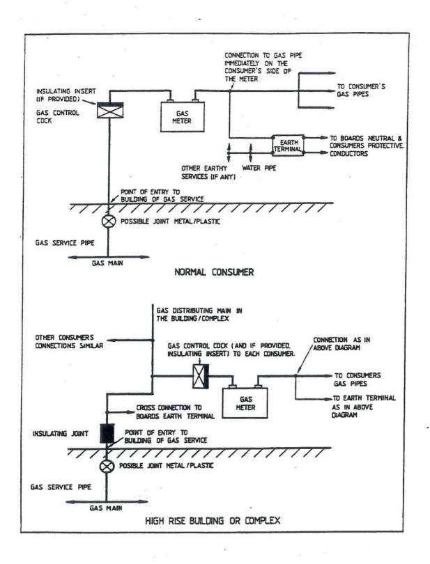
FIGURE 8: METHOD OF BONDING GAS SERVICE PIPES TO MAIN EARTH TERMINAL
