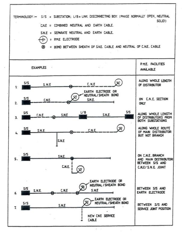
FIGURE 6: TYPICAL APPLICATIONS OF C.N.E. CABLES
