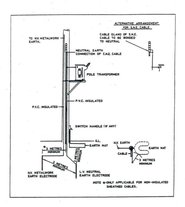
FIGURE 2: POLE TRANSFORMER FEEDING UNDERGROUND CABLE
